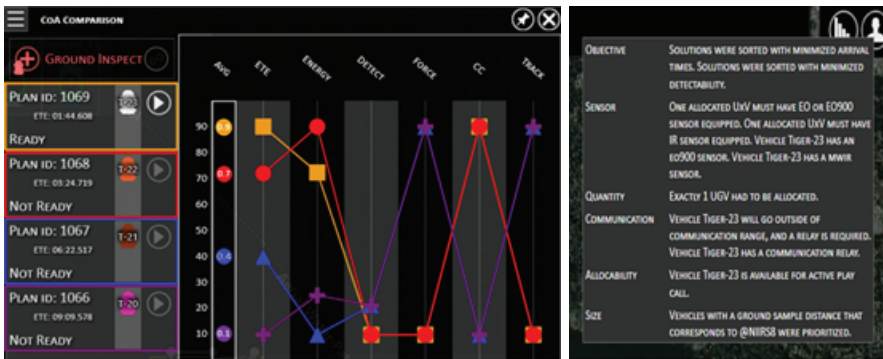
Figure D.2. AS-generated plans. Left: Plan Comparison HMI shows trade-off of several candidate AS-generated plans for a play. Right: AS's additional rationale for its recommended play plan.
