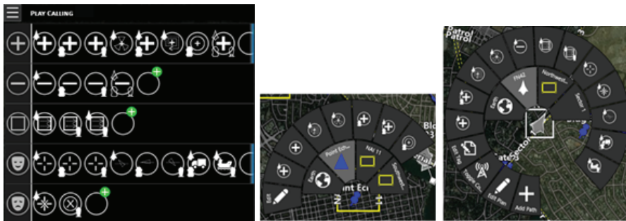
Figure D.1. Three HMIs to specify play and unmanned vehicle type with mouse or touch. Left: All base defense plays, including surveillance of a location, road, or area and others involving friendly or unfriendly entities (e.g., overwatch, escort, shadow, and cordon). Center: Radial menu pop-up includes only the play options relevant to the map location selected (i.e., no sea vehicle for land location). Right: Radial menu pop-up includes only the play options relevant to the vehicle selected on the map.
